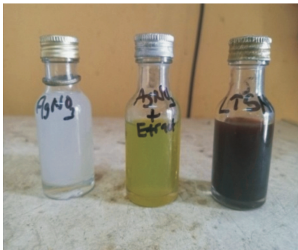
Figure 3.1. Visual observation of a.) Silver Nitrate solution b.) \text{AgNO}_3 and extract, and c.) Lactuca taraxacifolia nanoparticle
